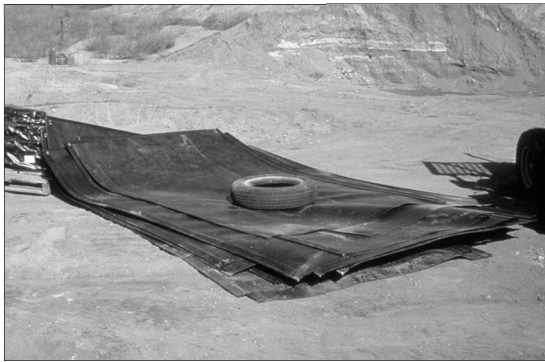
HDPE Sheet Piling
