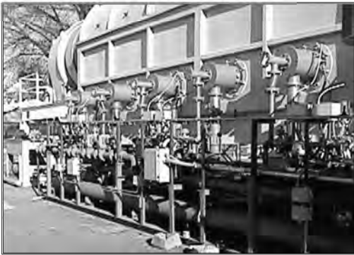
Burner Train Within Shroud
