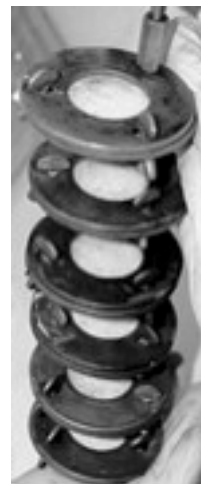
Figure 12-2. Array of POCIS on support rod ready for deployment in a protective canister
