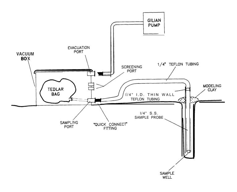
Figure 1: Sampling Train Schematic SOP #2149
