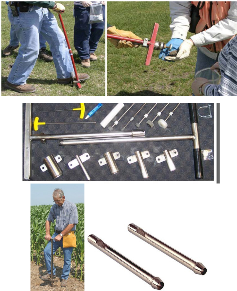
Figure 5-2a. Examples of coring devices for nonvolatile soil increment collection. Top to bottom: Multi-Incremental Sampling Tool (MIST™), EVC Incremental Sampler, JMC Backsaver Handle, and Soil Tube. , ITRC 2012.
