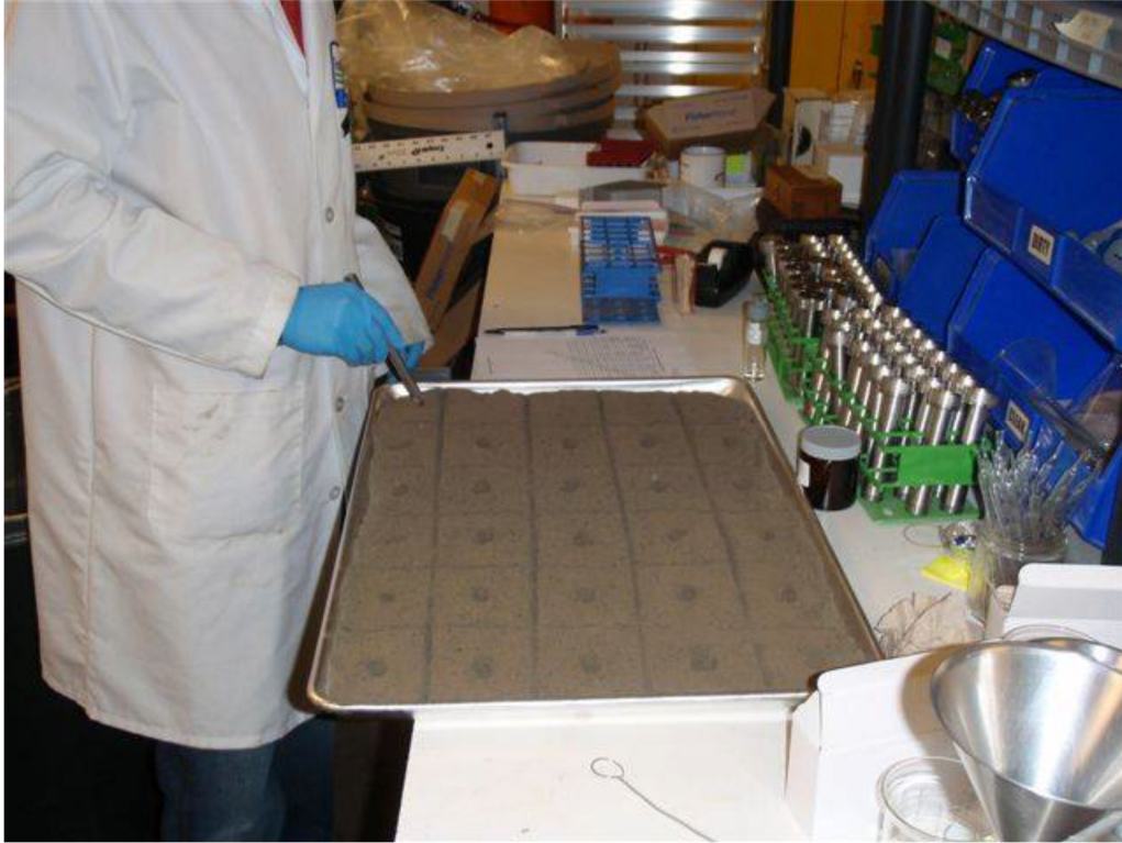
Figure 6-3. Example of 2-D Japanese slab-cake incremental subsampling on dried and sieved soil. ITRC, 2012
