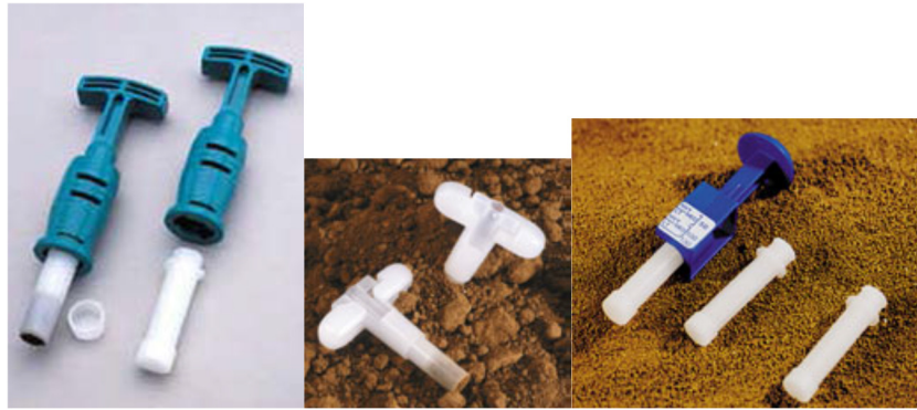
Figure 5-12. Examples of coring devices for VOC soil increment collection. Core N' One™ tool (left), Terra Core Sampler (center), and Easy Draw Syringe® and PowerStop Handle® (right). Source: Courtesy www.ennovativetech.com , ITRC 2012.
