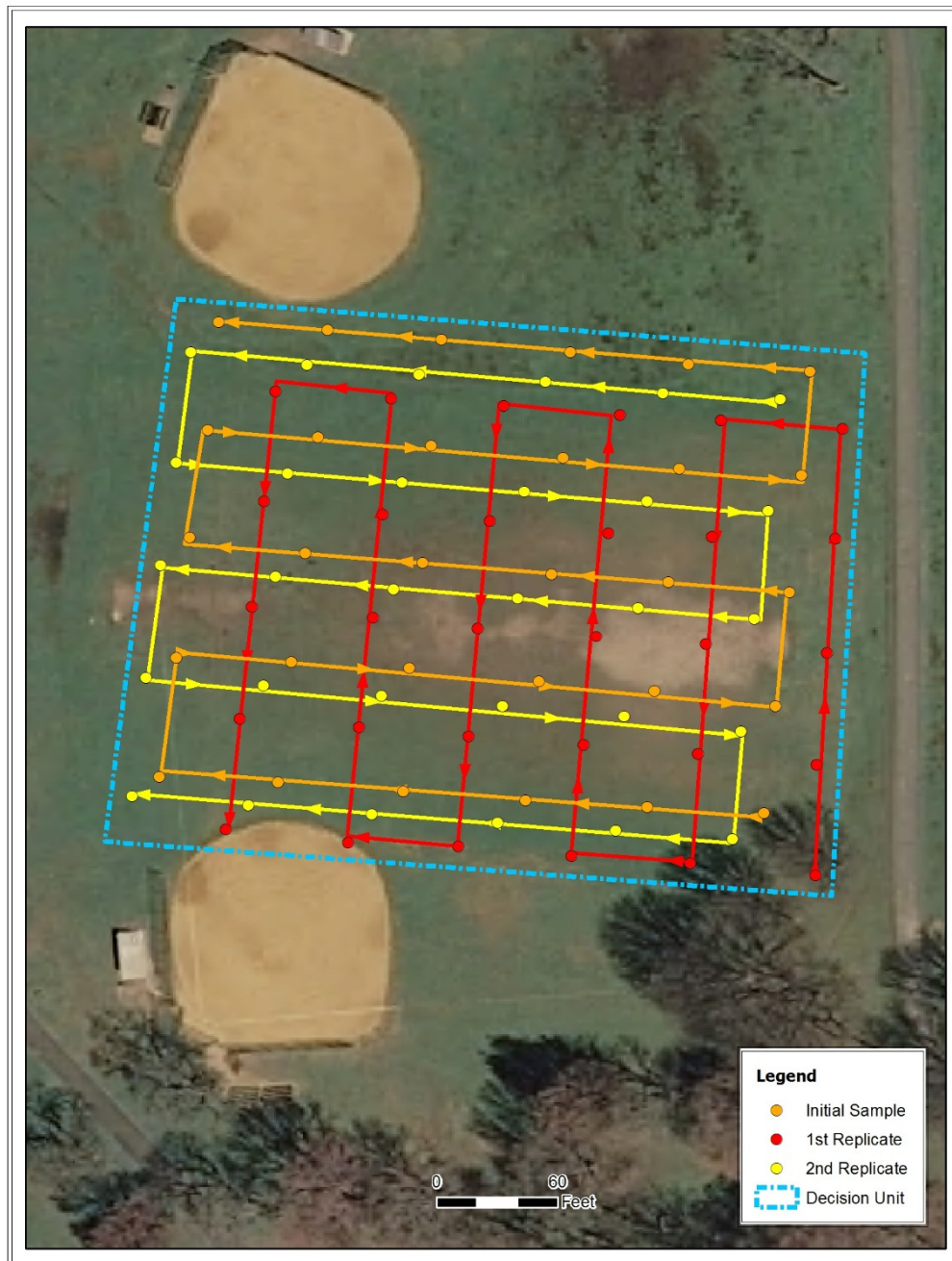
FIGURE 4. Collecting Replicate ISM Samples from a Decision Unit
