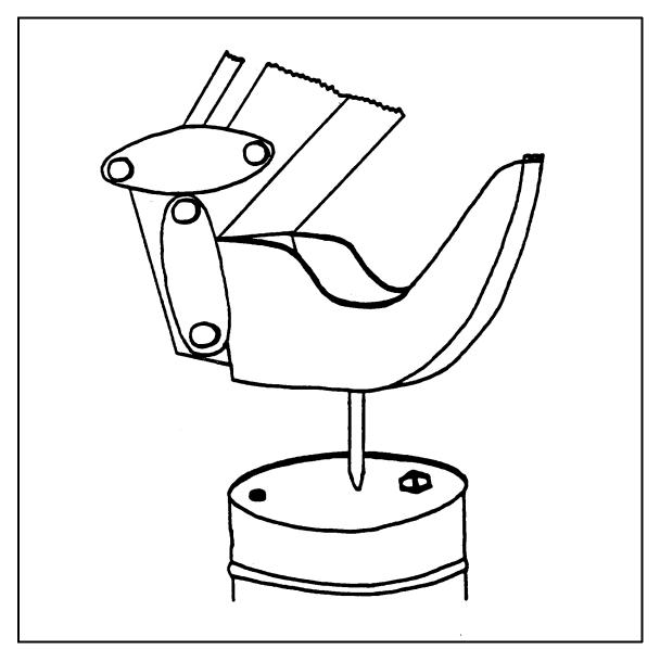
Figure 5. Hydraulic Drum Opener
