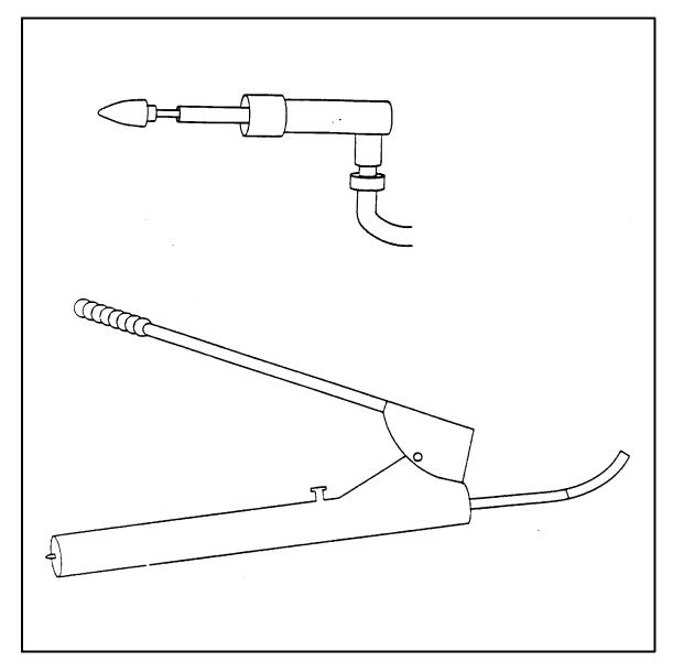
Figure 6. Pneumatic Bung Remover
